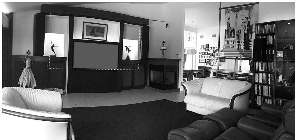
FIGURE 7.21 The author's entertainment/family room in California. The large L & R Revel Salon2s with bases removed are inverted so that the sound is perceived to originate at the bottom of the units. The physical locations of the loudspeakers and the ventriloquism effect provide excellent sound and picture correlation. There is a 65-inch flat screen TV and a motorized 10-foot front-projection screen shown by the dotted lines. The panoramic photograph distorts perspective; the true floor plan is in Figure 8.22.
